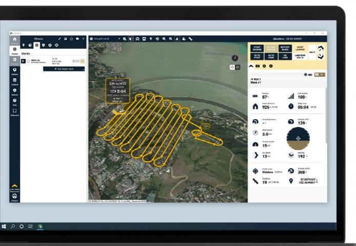
With eMotion, flights are built using mission blocks. Just choose your block, highlight the region you want to map, define key settings, and eMotion auto-generates your drone's flight plan. Multi-flight missions are supported and you can activate/import elevation data for even safer, terrain-accurate flights.
