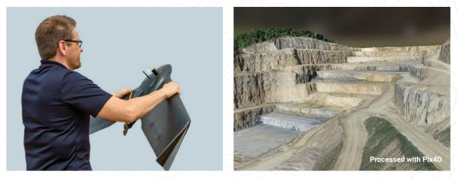
Upload your flight plan wirelessly to your drone. After a simple hand launch, your eBee X drone will then fly, capture images and land by itself.
