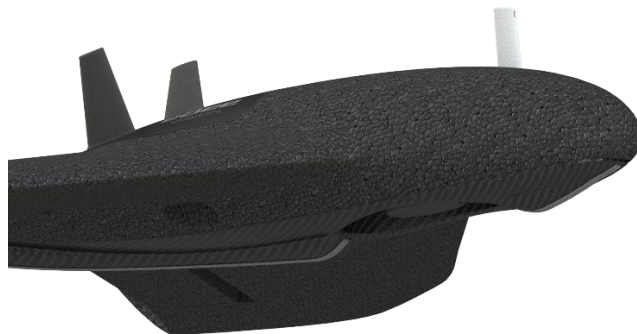
eBee VISION with folded (secured) gimbal
